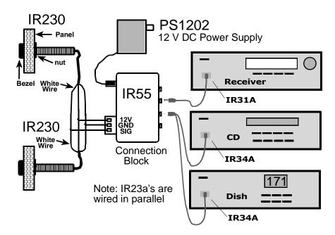
7. Now, plug in the PS1205 for up to ten infrared receivers.
